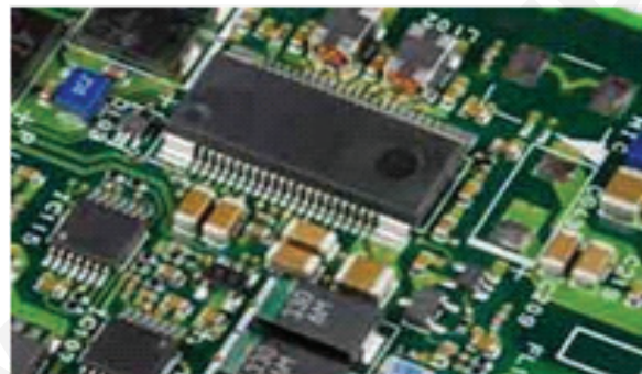
ICS WERE SOLDERED IN PCB BOARD
